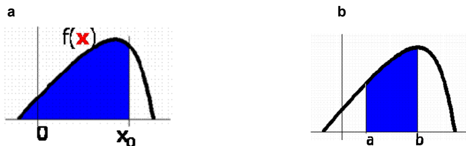
Figure 3.3. Probability density functions. a. In blue, P(x \leq x_0) , b. In blue, P(a \leq x \leq b)
